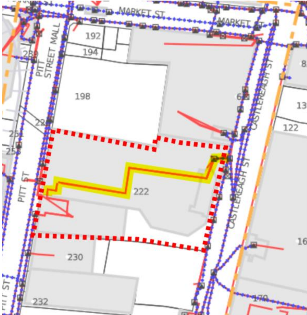
Figure 5: Optus existing Communications Services adjacent the site
